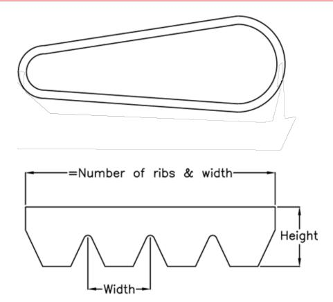
$\begin{array}{ll} \text{Datum Llength} = 1752 \\ \text{Height} &= 3.5 \\ \text{Number of ribs} = 7 \\ \text{Pitch} &= 2.34 \\ \end{array}$
